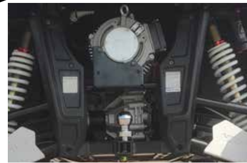
Air-cooled AC Asynchronous Motor and Controller Separation
